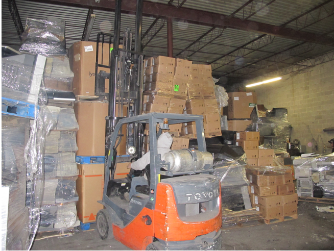
Attachment 7. Three photos showing unsafe stacking of heavy Equipment.
